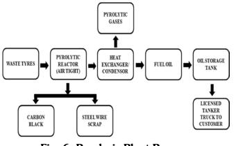
Fig. 6: Pyrolysis Plant Process
