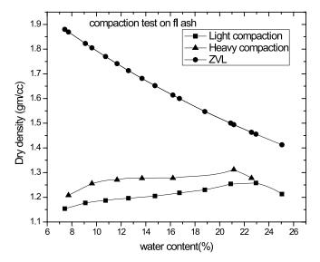
Fig. 8: Compaction Test on Fly-ash
