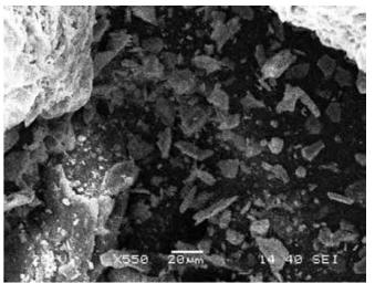
Fig. 5 Scanning Electron Micrograph of Shale
