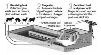
Fig. 2: Producing Electricity from Methane
