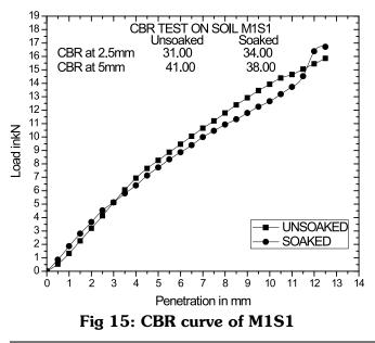
less than unsoaked CBR.CBR value found to be vary from 22.8 to 63.0. Hence as per IRC 37 the mix with more than 4% cement can be used for sub base. The mix without cement can be used on subgrade.
