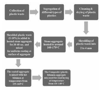
Fig. 3: Process Flow Diagram of Plastic Coated Bitumen Mix
