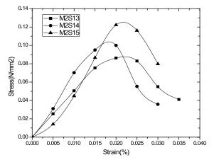
Fig. 14: Unconfined Compressive Strength Curves of different soil sample without cement
