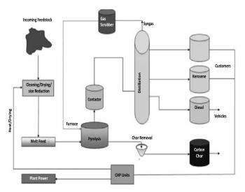
Fig. 6 Waste Plastic Pyrolysis Process System
