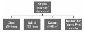
Fig. 7: Outputs of Pyrolysis Process
