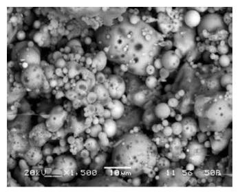
Fig. 6: Scanning Electron Micrograph of Fly-ash
