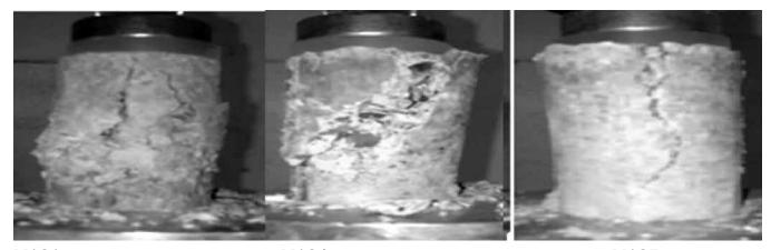
M1S1M1S4M1S7Fig 13: Typical Failure Pattern of Soil Samples M1S1, M1S4, M1S7 in UCS test
