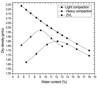
Fig. 9: Compaction Test on Shale
