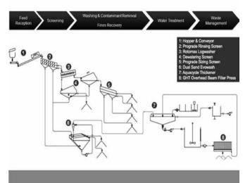
Fig. 2. Wet Processing of C&D waste
