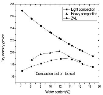
Fig. 10: Compaction Test on Top soil
