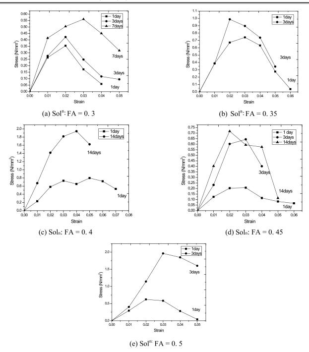
Fig. 1. Compressive Strength of Geopolymer Based Fly-ash of Different Ratios
