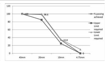
Fig. 6. Particle Size Sieve Analysis (Coarse Aggregate – 20mm nominal size) (b)Coarse Aggregate (RCA)
